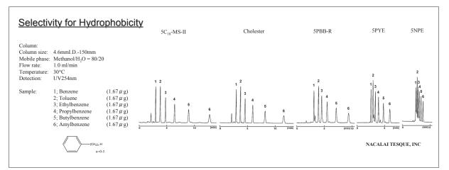
Lower concentration of organic solvent in mobile phase leads to much retention in reversed phase chromatography. In case of NPE, when methanol concentration is reduced to 60%, the retention times increase to those similar to C<sub>18</sub> with 80% methanol.
