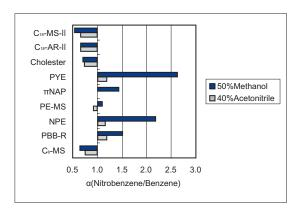
The graph of selectivity for polar functional group is shown below. Among nine COSMOSIL columns, PYE and NPE columns have the highest selectivity factors for polar groups. As to mobile phases, methanol is more effective than acetonitrile for separation using  $\pi$ - $\pi$  interaction.
