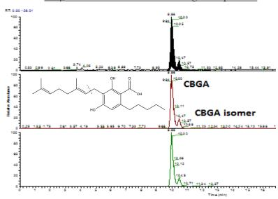
HPLC Column: COSMOCORE Cholester 2.1 mm ID x 100 mm, 2.6 μm
