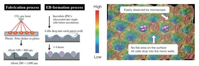
EZ SPHERE is a unique micro-fabricated plastic vessel and very useful for mass-production of EBs with uniform size.
