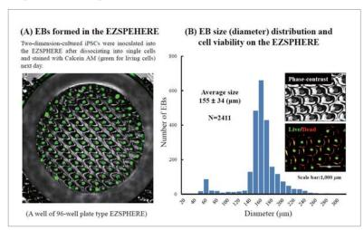
Fluorescence microscopy image of EBs obtained on the EZSPHERE (A). EBs created on the 35 mm dish type EZSPHERE were imaged and analyzed with the digital image analyzing software "Image J" to determine size distribution. Histogram of EB size (diameter) distribution. Fluorescence microscopy revealed that the almost EBs were alive with uniform size (B).
