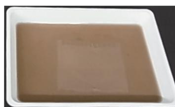
Gel : TGX gel from Bio-rad (W 86 mm × L 70 mm × H 1 mm)
